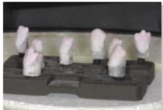
Figure 26: Fired refractory dies.
